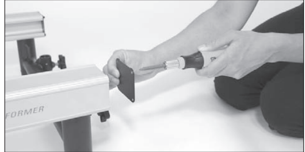
6. Using a Phillips screwdriver, replace stopper plates.
